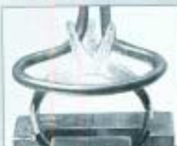
Platinum Setting 5 second solder time.
